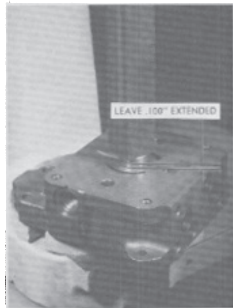
FIG. 82. Install second Needle Bearing
