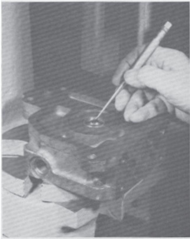
FIG. 79. Remove Seal Retainer "O" Ring
